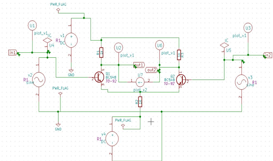
Figure 1: BJT based Differential Amplifier
