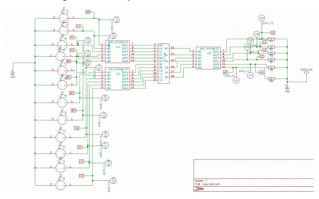
Here I used a subcircuit for four bit carry save adder. The internal structure of carry save adder is shown below.
